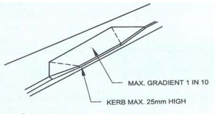
FIG. 1 SUITABLE METHOD OF BLENDING PAVEMENT AND ROADWAY SURFACES
