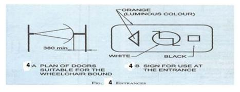
(b) At least one entrance usable by individuals in wheelchairs shall be on a level that would make the elevators accessible.
